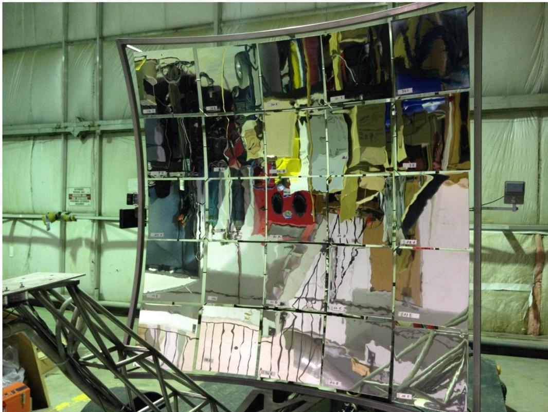
**Figure 1: SHEC's Prior Technology - Glass Parabolic Mirror**
